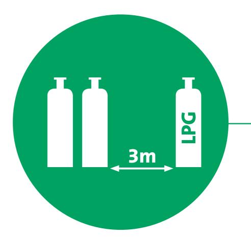
Segregate cylinders by the properties of the gas ensuring that LPG is separated from all cylinders by a minimum of 3 metres (or a firewall)
